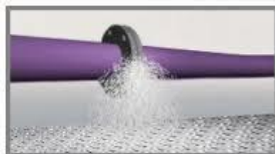
Unprotected leaking flange
